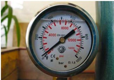
(e) the vertical stress measuring gauges
