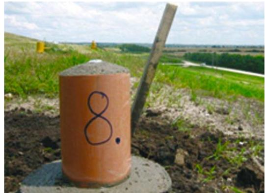
Figure 5. Settlement measuring point.
