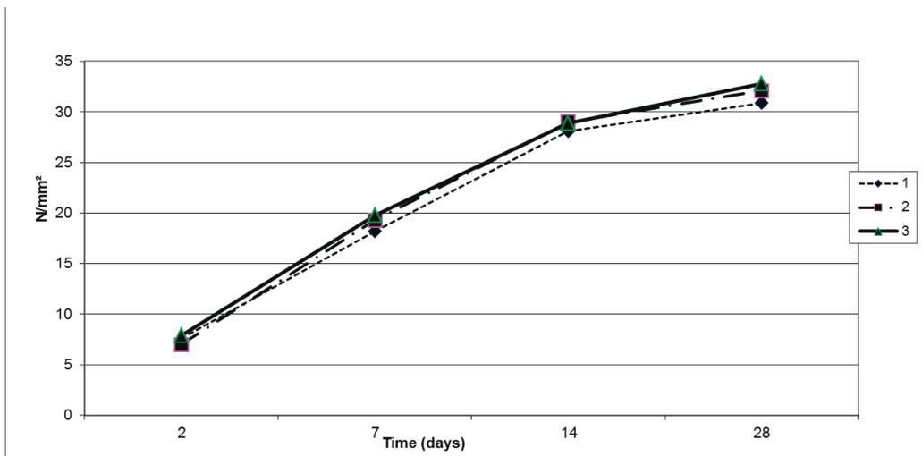
Figure 9. Values of compression strength ( 1- NC, 2-LC1, 3-LC2)
