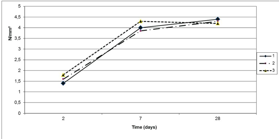
Figure 8. Values of tensile strength ( 1- NC, 2-LC1, 3-LC2)
