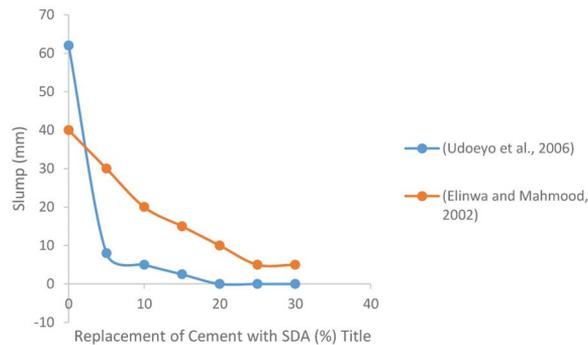
Figure 4. Slump characteristic of concrete specimens with SDA [37, 53]
