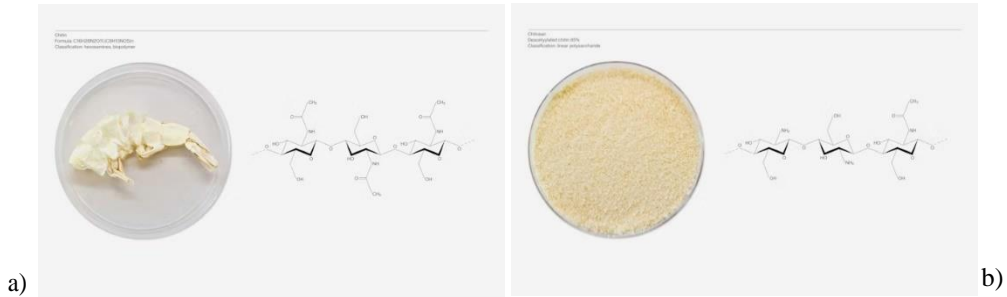
Figure 5. a) Shrimp-shell derived chitin b) Dried chitosan derived from chitin, Oxman projects.
